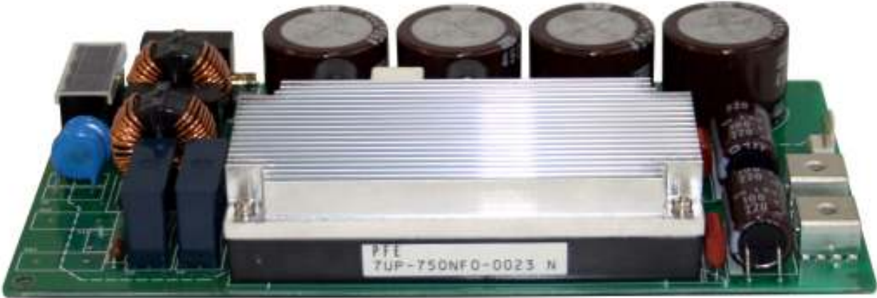
PFE Series Power Module mounted on Evaluation Board with heatsink and external components
